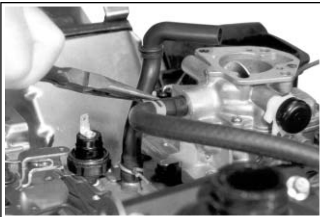
Figure 9-12. Disconnecting Fuel Inlet Line at Carburetor.
